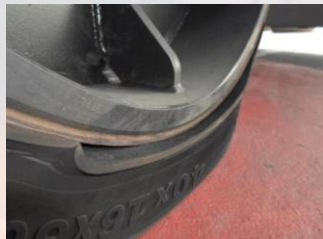
Steel band debonding
